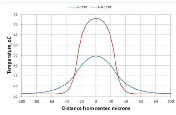
**Figure 1. Temperature of 50micron cylindrical object heated with pulse with width of tree times longer than TRT and 3 times shorter of TRT.**
